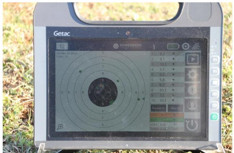
Portable wireless receiver behind the firing line
